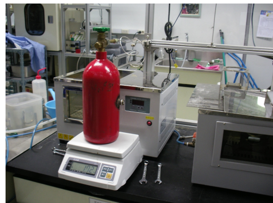
Figure 2. Picture of charging CO 2 into the extinguisher.
